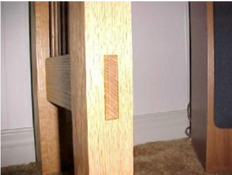
**Of** course the tiny 3/8" tenons of the spindles will not be difficult to cut and fit, but most of the time I test each tenon for fit as I cut them. I usually determine which piece will go where before I begin my joinery cuts - making the decisions based on grain and overall appearance of the wood. Knowing how everything will fit together gives you the
