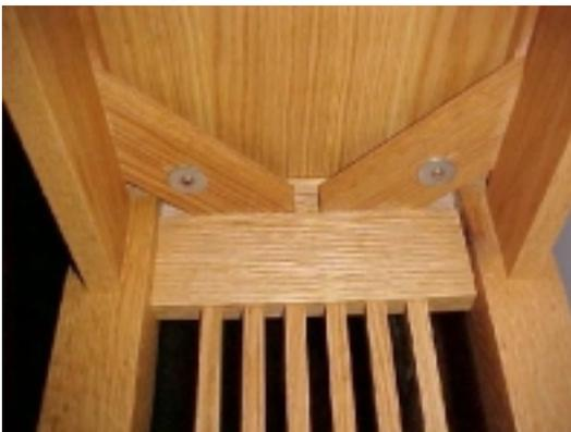
**Mortise** and Tenon joints were used for the lower end rails, but I chose to use biscuits to attach the upper side and end rails to the legs. With the addition of inside corner braces glued into dados on the insides of the rails, the biscuits are plenty strong enough to hold everything together. These corner braces serve two purposes: they help hold the whole
